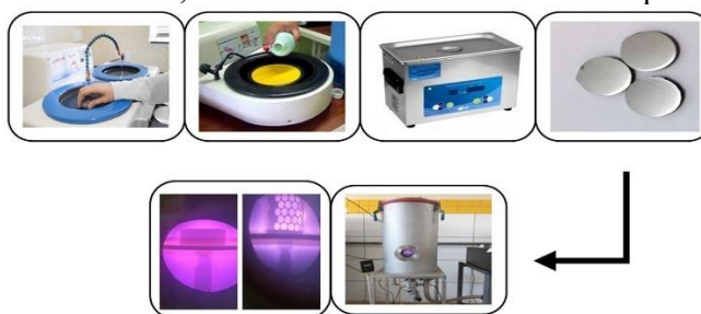
Fig. 1. Process for film deposition on NiCr samples.
