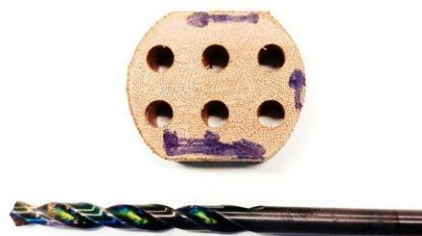
Fig. 2. Drill and drilling finished in Celeron polymer.
